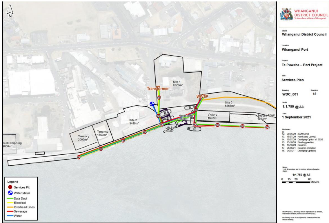
Figure 8: Proposed locations of services associated with transformer and WWTP (supplied Whanganui District Council)
