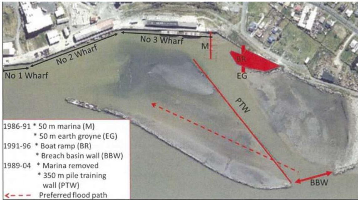
Figure 10: Locations of wharves and more recent structures in the CMA (supplied Whanganui District Council)
